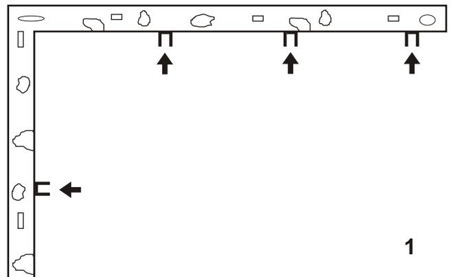
2. Lift the partition walls into vertical position and fasten them to the aluminium profiles by using 4 x 20 screws. Place 100 -120 mm high supports below the elements at the front edge.
